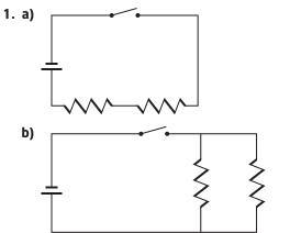
**2.** If one bulb burned out, the circuit would become open and the other lights would go out.
