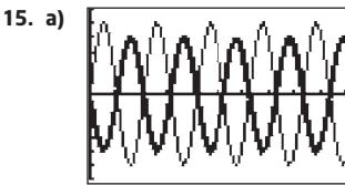
b) The maxima and minima are located at the same x-coordinates. This will result in destructive interference.
