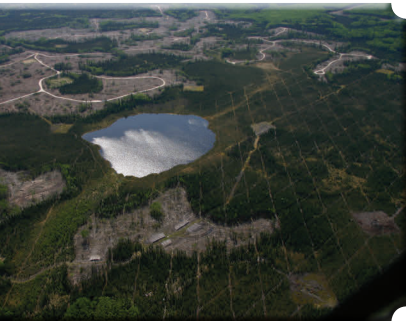
Figure 4-14 The exploration sites and lines cut through the boreal forest shown in this aerial photograph are in northern Alberta. To locate and map underground oil sands, companies cut a grid of lines. The grid enables geophysicists to bring vibrator and recorder trucks into the forested areas so they can take measurements.
