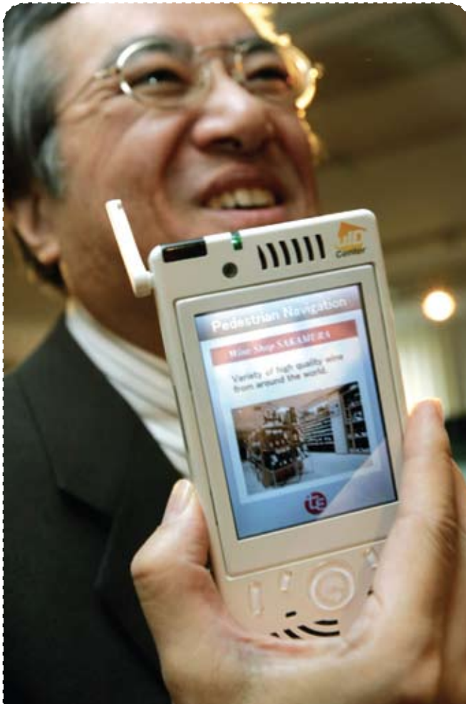
Figure 11-4 A Japanese man holds a portable device with an earphone plug and a screen as he participates in testing the Tokyo Ubiquitous Technology Project in March 2007. The $8.7-million (U.S.) project, which is supported by the Japanese government, involves sending messages to shoppers from 1200 computer chips lodged in lampposts, subway station ceilings, and sidewalks. The messages contain maps, store guides, and quick history lessons. How might this use of technology reinforce national interest rather than internationalism?
