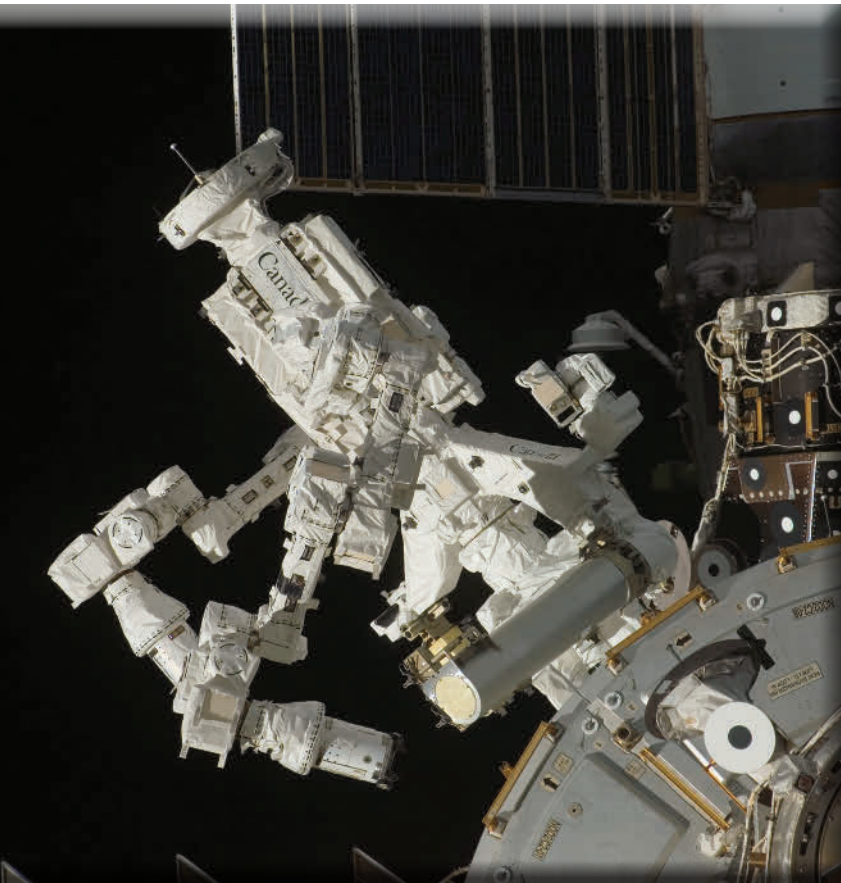
Figure 15-19 Dextre, the robot developed by MacDonald, Dettwiler and Associates in partnership with the Canadian Space Agency, cost $200 million and was installed on the International Space Station in March 2008. Dextre can lift nearly 600 kilograms, is capable of sensing the movements of the objects it manipulates, and is expected to perform important tasks in maintaining the station.
