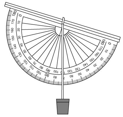
**3.** When trying to determine the measure of an object that is too tall to measure directly, look through the straw to the top of the object that you are measuring. Find a horizontal line of sight. Find the angle measurement where the string and protractor intersect. To determine the angle of elevation, subtract this measurement from 90°.
