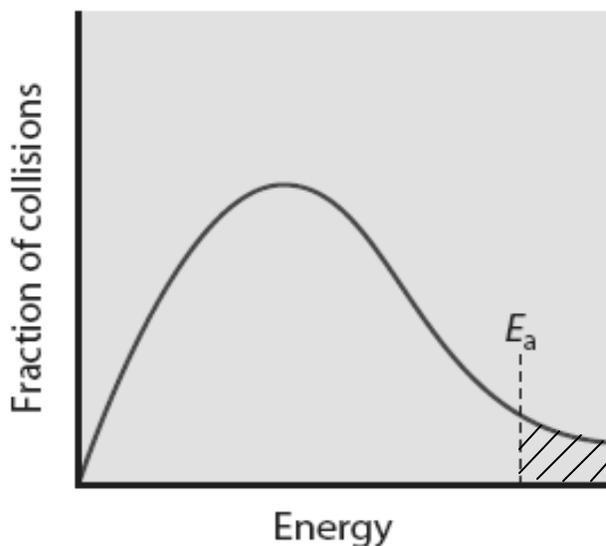
The area under a Maxwell-Boltzmann distribution graph represents the distribution of the kinetic energy of collisions at a constant temperature. At any given temperature, only a certain fraction of the molecules in a sample have enough kinetic energy to react.
