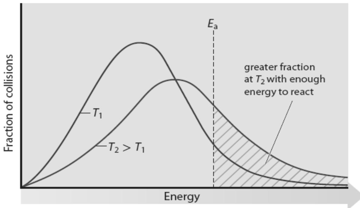
At increased temperatures, more particles collide with enough energy to react.
