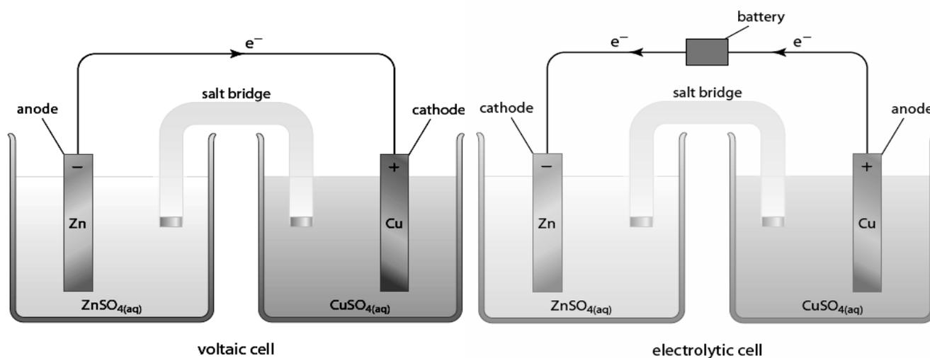
Adding an external voltage to reverse the electron flow converts a Daniell cell from a voltaic cell into an electrolytic cell.
