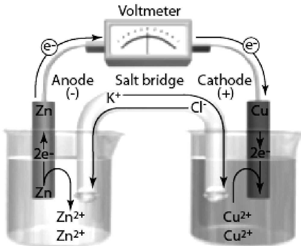
By convention, voltaic cells, such as this Daniell cell, are usually drawn with the anode, where oxidation occurs, on the left and the cathode, where reduction occurs, on the right.
