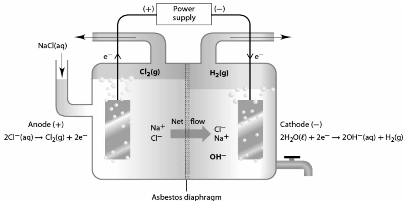
The chlor-alkali cell in this diagram electrolyzes an aqueous solution of sodium chloride to produce chlorine gas, hydrogen gas, and aqueous sodium hydroxide.
