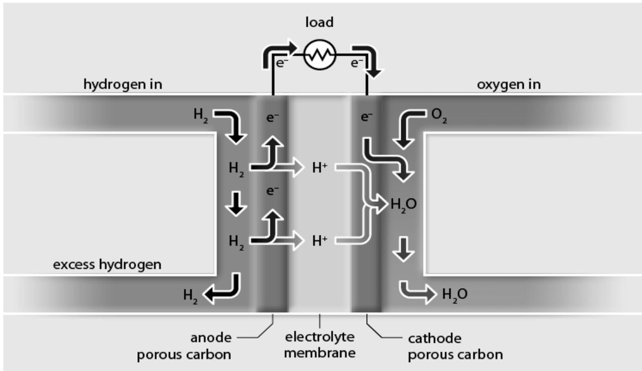
Hydrogen gas from tanks and oxygen in air provide a continuous supply of fuel for the fuel cell. The electrolyte is a solid polymer that allows hydrogen ions to pass through.
