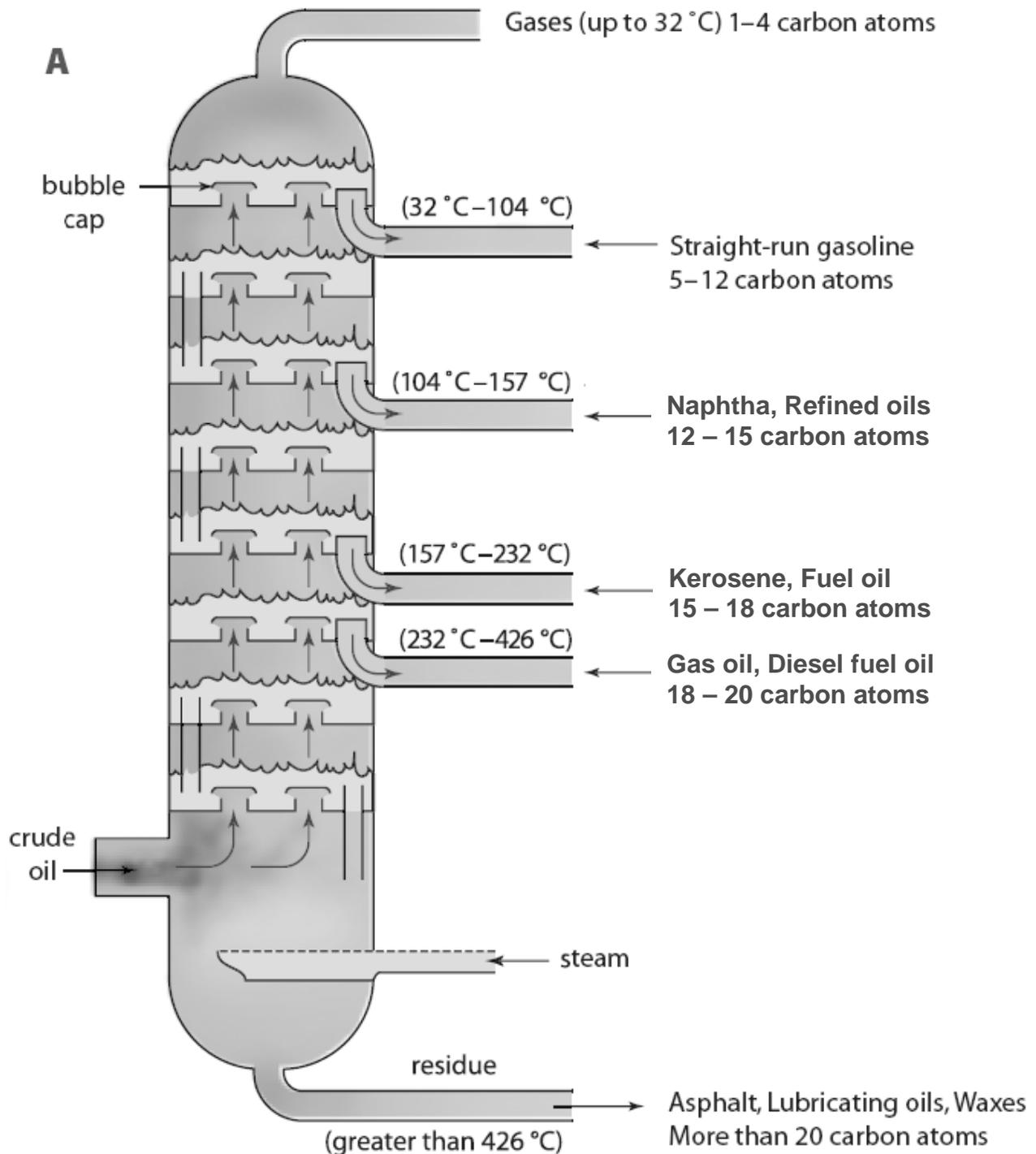
Fractional distillation involves successive heating, evaporation, cooling, and condensation. Fractional distillation towers can be as high as 60 m.
