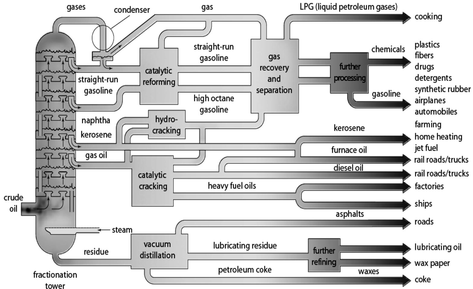
Notice the terms *catalytic reforming*, *hydrocracking*, and *catalytic cracking*. Each of these is a different process, but they all change the structure of some of the hydrocarbons into more useful products.
