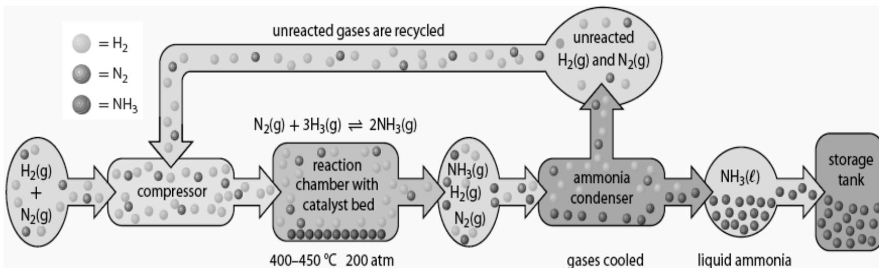
The catalyst that is often used with the Haber-Bosch process, shown in the diagram, is a mixture of  $\text{MgO}(\text{s})$ ,  $\text{Al}_2\text{O}_3(\text{s})$ , and  $\text{SiO}_2(\text{s})$ , with embedded iron crystals.
