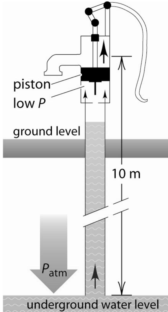
The pump creates a partial vacuum in the pipe and the atmospheric pressure pushes water up the pipe. Atmospheric pressure can push water up to a height of only 10 m.
