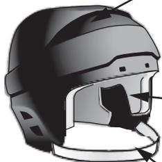
**Shell:** The shell of a hockey **helmet** is made of impact plastic. The shell is designed to absorb and deflect the energy of a body check or a collision with the boards. It also protects the head from any puck or stick impact.
