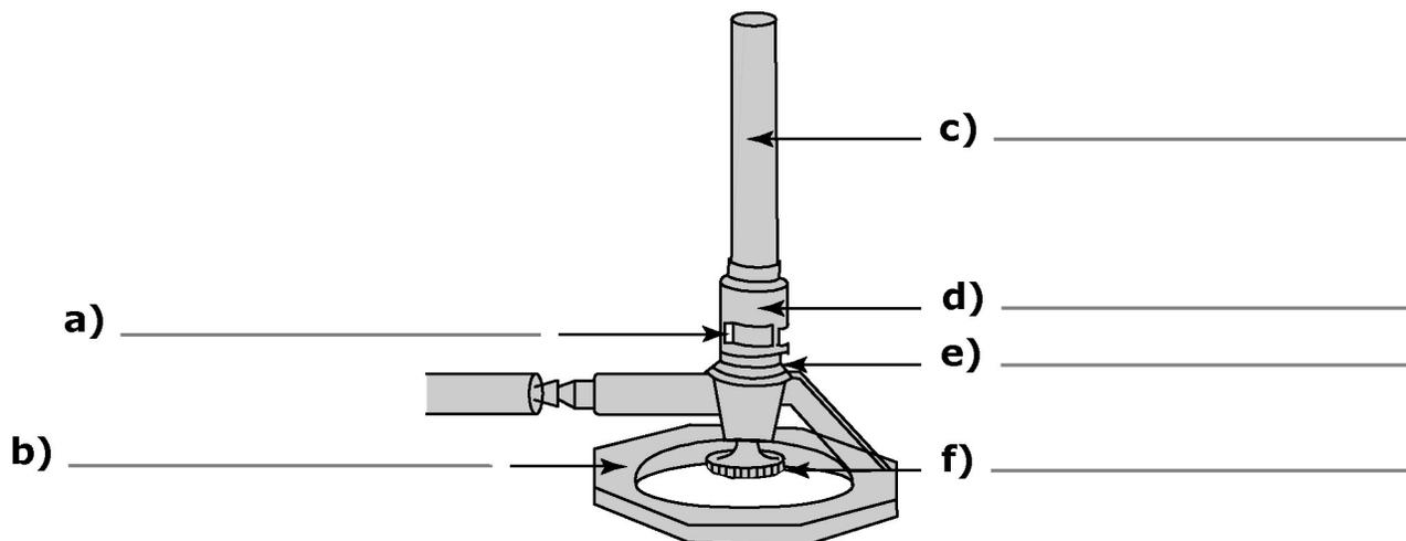
A Bunsen burner has inlets for gas and air. A proper balance of each is needed to produce a suitable flame and to ensure the gas burns completely.
