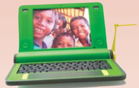
Figure 3-4 Because the display screen has fewer colour filters than normal, the 2B1 children's laptop uses just 2 watts of power compared with the 25 to 45 watts required to power a conventional laptop. Each 2B1 has its own antenna and video camera lens.
