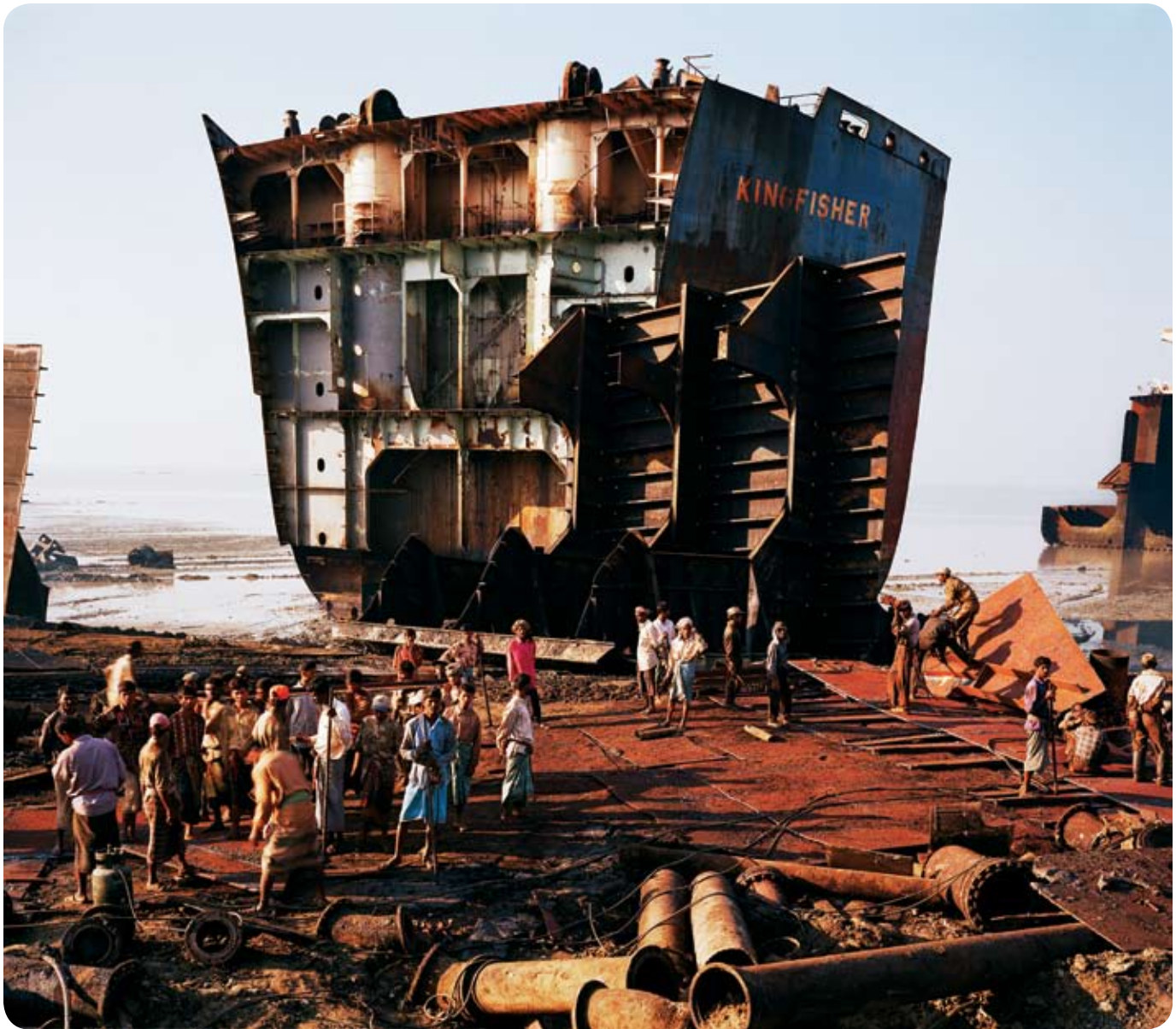
Figure 11-1 This photograph by Canadian Edward Burtynsky is titled Shipbreaking No. 4 . When ships become too old to be useful, they are sold to recyclers. Shipbreaking is big business in Bangladesh, India, China, Pakistan, and Turkey, where ships are run up onto beaches and dismantled. The steel and other materials are recycled and used in new products. But shipbreaking can have severe effects on the environment and on the health of the workers involved.
