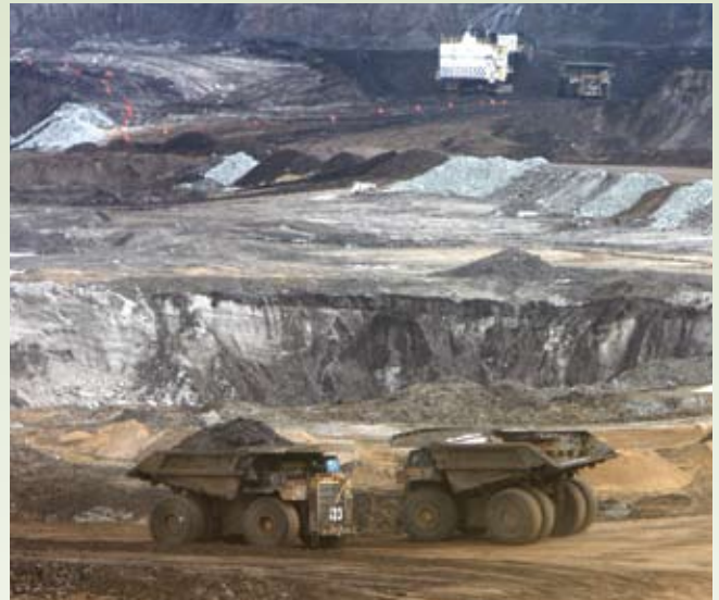
Figure 15-13 Huge trucks and machines extract earth from an open pit mine near Fort McMurray. Hot water is then used to separate the oil from the sand.
