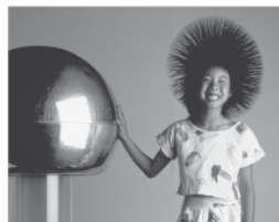
Figure 1.4 This machine creates a strong static electric charge on its dome. Each strand of hair on this student's head repels each of the other strands when she touches the charged dome.
