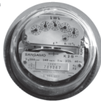
Figure 2.10 This is an electric meter. A technician can read the dials to find out how much electricity has been used since the last reading. Do you know where to find your home or building's electric meter?
