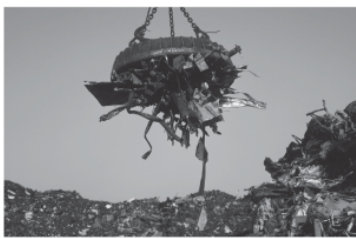
Figure 2.4 Electromagnets are used at scrap yards and recycling centres to pick up metals and separate them from other materials.
