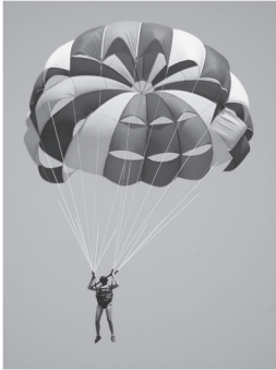
Figure 3.13 A parachute is designed to increase drag. This allows things to fall slowly.
