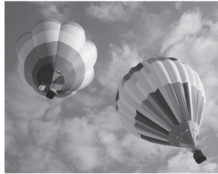
Figure 3.7 Ballooning is a balancing act. A balloon continues to rise until the forces of gravity and buoyancy acting on the balloon are equal.
