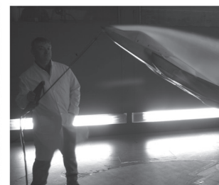
Figure 4.5 A wind tunnel shows how air moves around and over a solid object.
