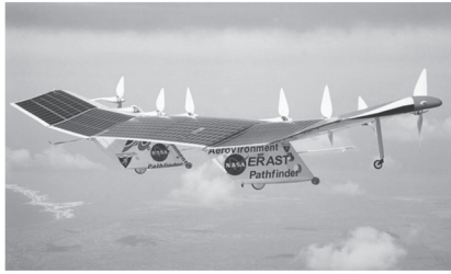
Figure 4.3 This plane has a specialized function: to fly using only the Sun's energy.
